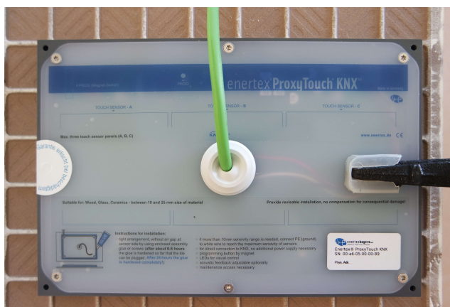
Figure 3: Fixing the housing
